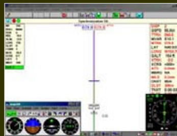
Figure 4: Screen with flight lines used by the aircraft pilot during flights. Each photograph is geo-coded, and stamped with date and flight altitude.
