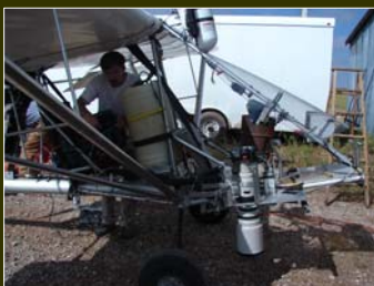
Figure 2: Close up of aircraft. Note digital cameras in the foreground. Sam Cox is programming flight lines on one of the 2 on-board laptop computers.
