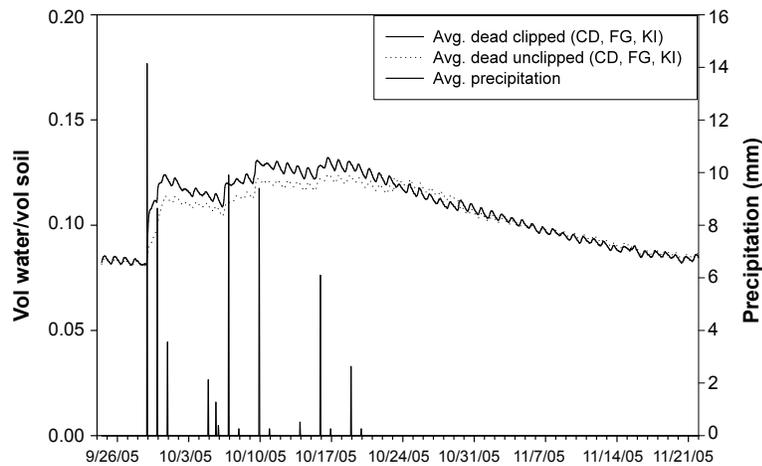
**Figure 2**—Soil volumetric water content response to rainfall under clipped and unclipped herbaceous vegetation beneath dead trees in CD, FG, and KI enclosures at the Corona Ranch.
