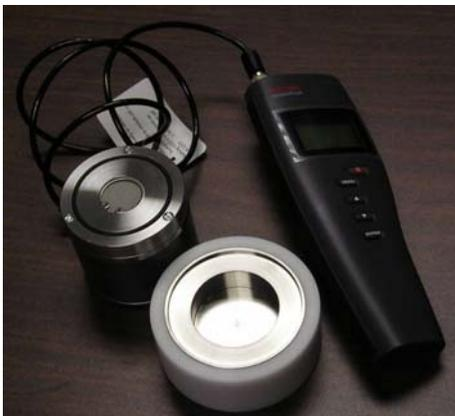
Rotronic, Inc. offers three series of water activity meters: hygropalm Aw, hygrolab 2, and hygrolab 3. All of these meters determine Aw in as little as 5 minutes. The Hygropalm Aw is recommended for smaller jerky processors with an accuracy level of 0.015 Aw. It uses an integrated circuit humidity sensor. The approximate cost is \$ 2300.
