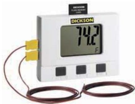
Data loggers are microprocessor units that both read and store data. In this case the measurement is temperature via one or two K-type probes. So, for example, both wet and dry bulb thermometer readings can be measured and logged into memory. When a run is complete the data can be transferred to a computer using several different methods.
