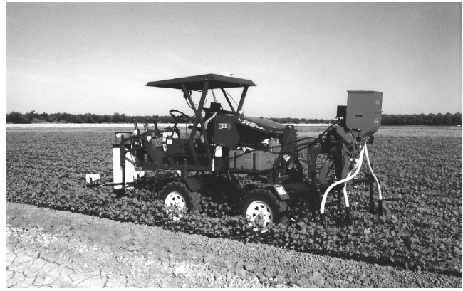
Figure 1. 4WD vehicle with IR, GPS, variable rate fertilizer applicator and insect vacuuming system.
