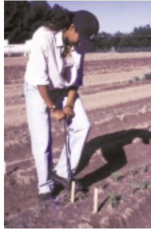
Figure 16. Collect soil cores with a soil probe.
