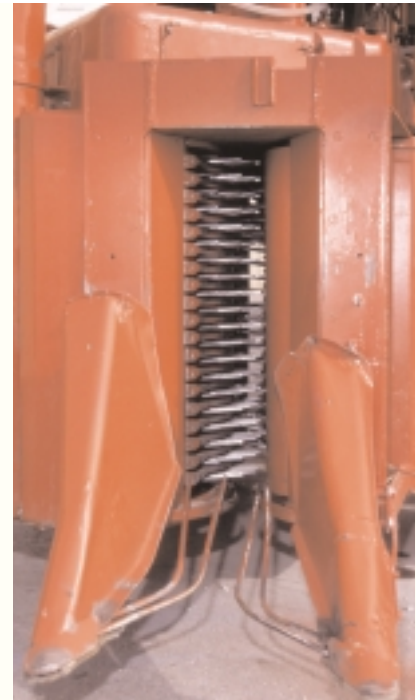
Picker perfect: Researchers are designing cotton picker spindles that are gentler on fiber.
