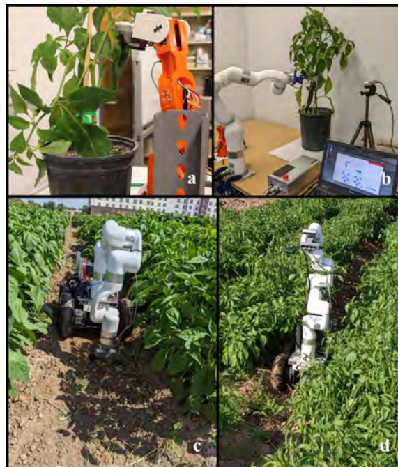
Figure 1: a) 5 degrees-of-freedom (DoF) robotic arm with a cutter end-effector harvesting green chile peppers in an indoor setting, b) a 6-DoF robotic arm with integrated wrist camera and an cutter end-effector identifies the location of the stem and harvests green chile peppers, c) robotic soil moisture and temperature measurements at the NMSU's Heritage field, and d) image capturing and visual remote sensing using an autonomous ground mobile robotic arm in chile pepper testing field at the NMSU's Leyendecker Plant Science Center
