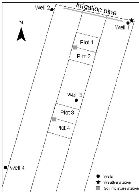
Figure 1. Schematic layout of the deep percolation study site at the Alcalde Science Center.
