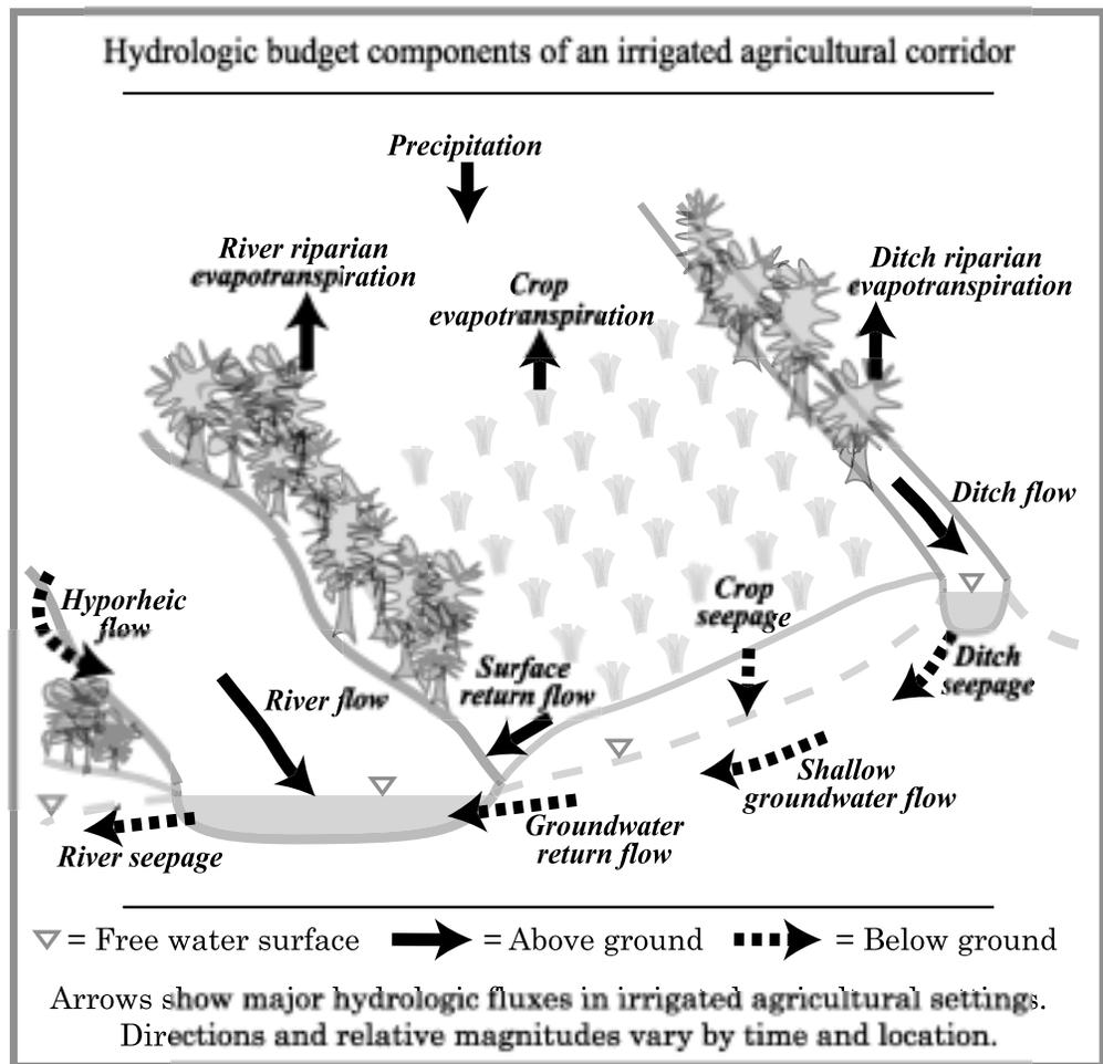
groundwater recharge and groundwater return flow to the river. The scenario presented here is intended as an illustration of the existence of multiple flow paths, and it should be recognized that directions, rates, and volumes of water moving through each path vary by time and location.
