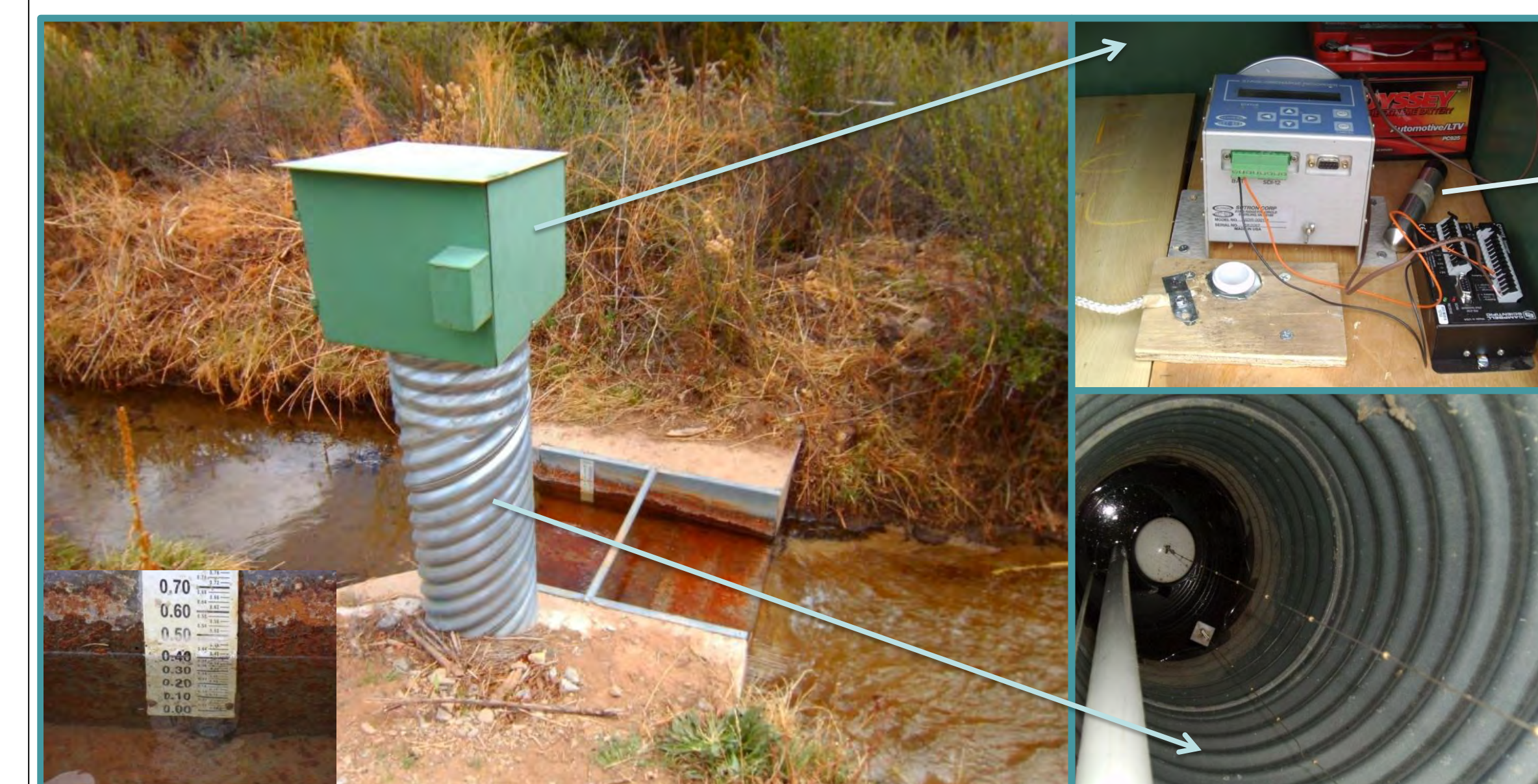
A flume used to measure surface water discharge automatically (Above Left/Inset). A Stage Discharge Recorder (SDR) and data logger are used to record data automatically (Above Top Right). Inside of the stilling well; SDR float and cable (Above Bottom Left)
