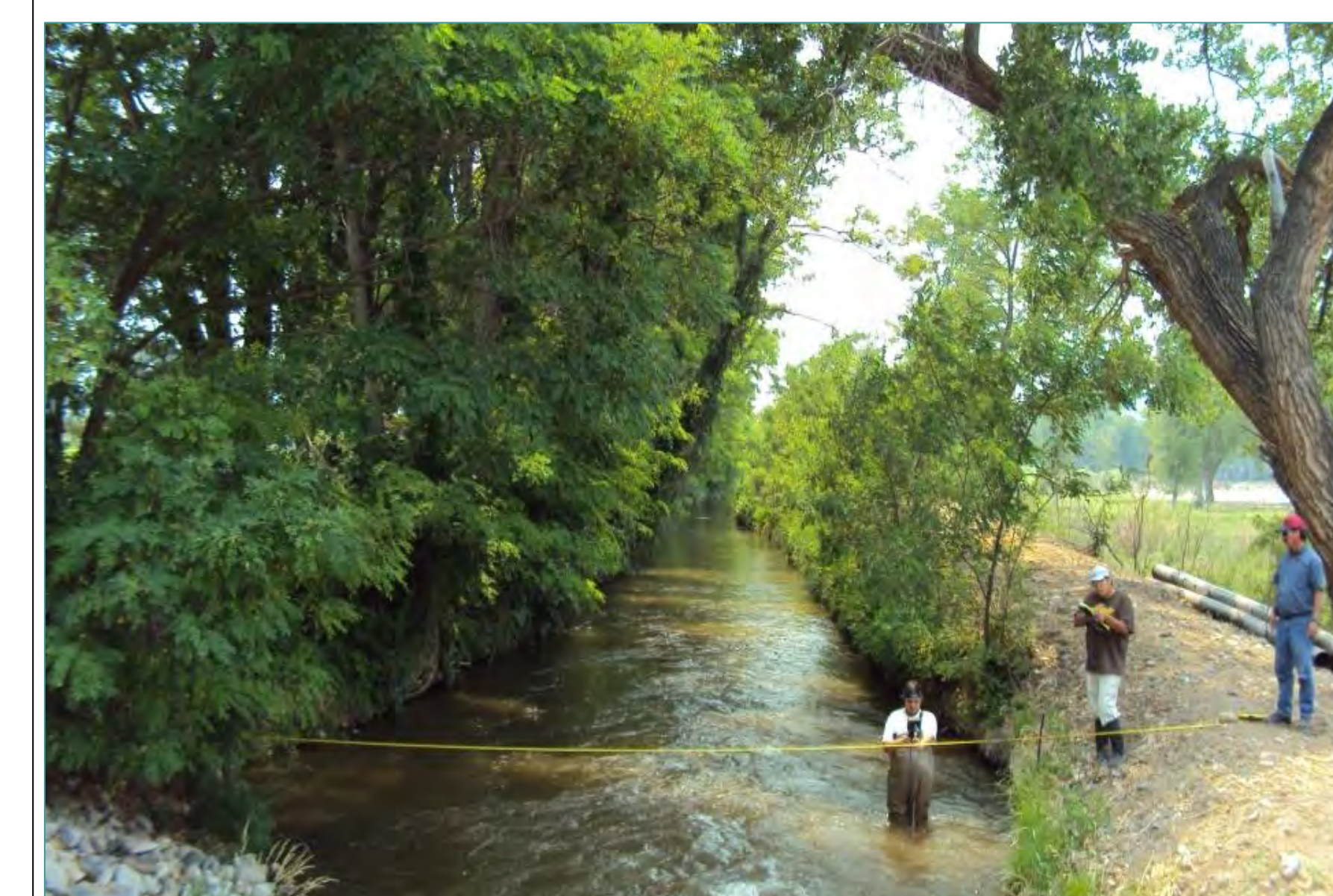
Acequia flow measurements being taken in Alcalde, NM
