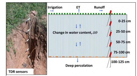
• A daily water balance method was used for determining deep percolation below the top 1-m soil.
