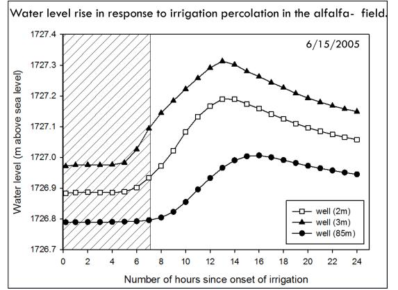
• Time of response and water table rise were different at different well distance from the irrigation line.
