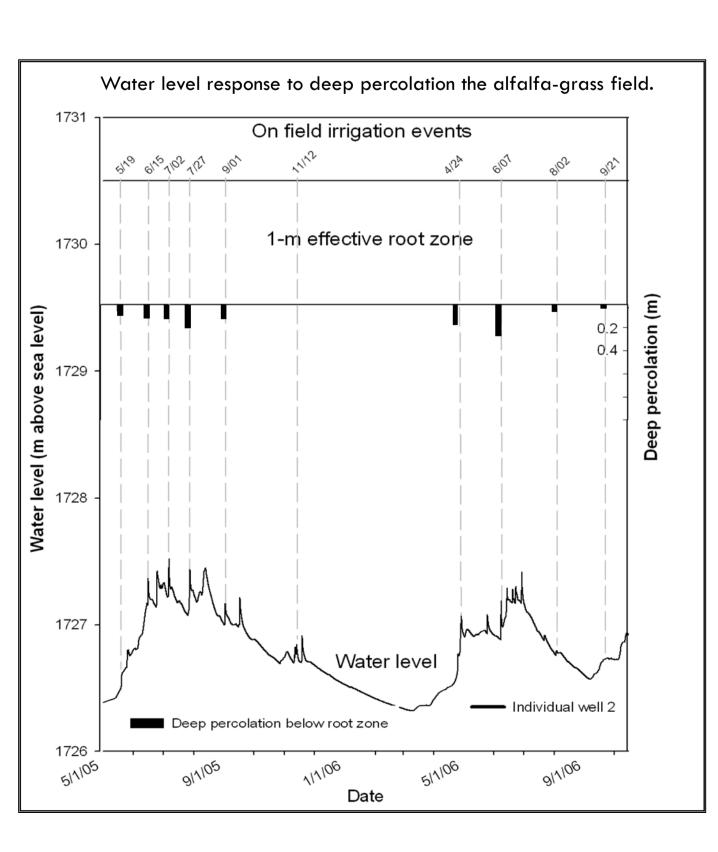
• A transient water level rise was observed in response to deep percolation from irrigation.
