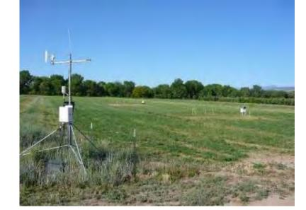
• Weather data collected on-site was used for calculating crop ET.
