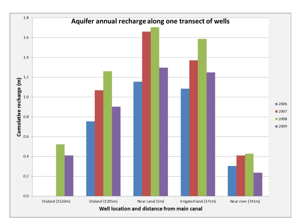
• A monthly step water level fluctuation method was used to calculate cumulative annual recharge at different well locations. Higher shallow aquifer recharge in transect 1 occurred in the well located near the main canal.
