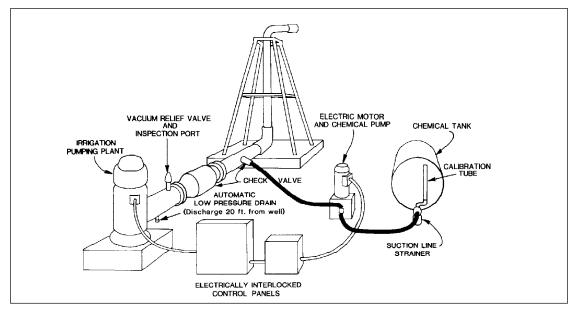
Figure 3 : Chemigation system with backflow prevention for a center pivot sprinkler.
