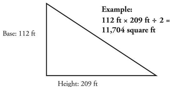
**Triangle shapes with no square corners:** Create right angles by choosing a transverse line and measuring the length of the new side. Include the new lines in your field drawing.
