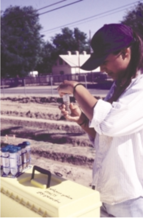
Figure 19. Add soil sample to the tube.
