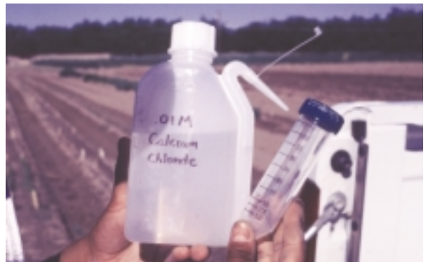
Figure 18. Fill centrifuge tube with calcium chloride.
